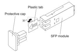
Figure 28. Unlocking the SFP module latch - plastic variety
